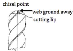
Figure: standard twist drill terminology
